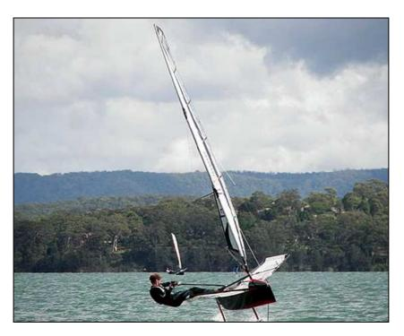
When sailing upwind in light/moderate conditions, the bow should only be angled about 1-3 degrees up and the wand should be angled approximately 30 degrees perpendicular to the bow so that the front foil flap is neutral for the best efficiency.
