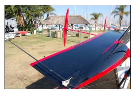
When the wand is pushed back as far as it can go (ie when the flap should be fully down), the wand should line up with the letters 'er' in the signage 'Bladerider' on the side of the hull (or be approximately 60 degrees to the bow as per photo below).
