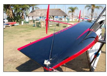
If the wand cannot be pushed back without force to the letters 'er' on the side of the hull (ie when the boat is sailed with the wand tip just under the waterline position), then there is probably too much lift on the front flap and boat will sail very high out of the water all the time. Therefore you will need screw in the socket joint head until you get the desired push-rod length and hence the correct amount of lift on the front foil flap (as per the photo below).
