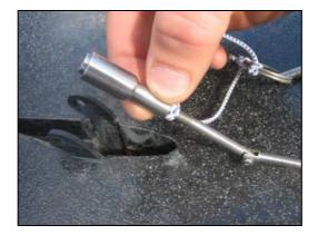
However if you have screwed in your ball/socket joint head all the way and you cannot thread it on any more, then you will need to remove and cut down the threaded push-rod adjuster by approximately 5mm. It is highly recommended that you do this in a locking vice and find a 5mm (nonnyloc nut) to thread on first before you start cutting, as so you can unwind this after you have made the cut, and it will clean the thread up for you (as seen below).
