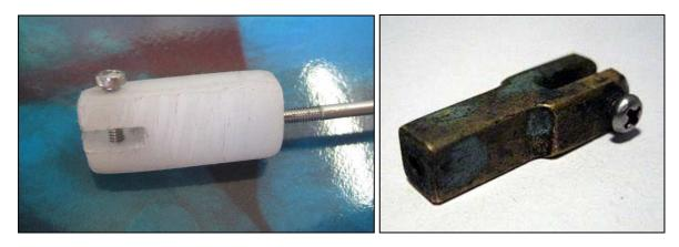
Alternatively, Bladerider now have stock supplies of a new fitting made from brass. Contact your reseller if you need one of these. All new centerboards from March 2008 will have these fitted as supplied.
